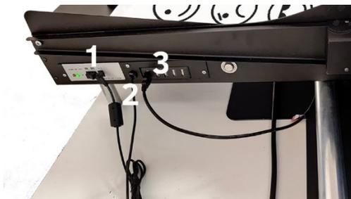
1. Connect adapter (next to sheet feeder ON/OFF switch)
