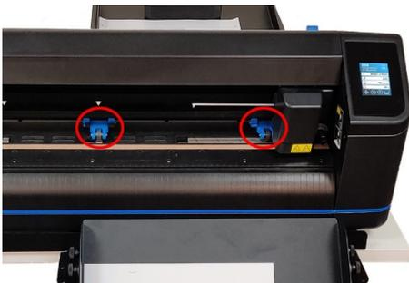
Position pinch rollers (left one fixed, right one adjust to sheet size)
