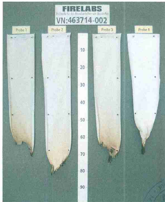
Fig. 4 View of test specimen after the test (sample 4: rear side)
