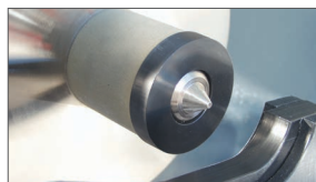
Pneumatic locking system of spindle
