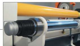
Front unwinding shaft with brake to rewinding log rolls
