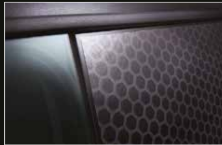
▲ Create a uniform relief cut between window graphic and rubber molding.
